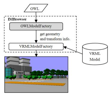
Fig. 5. Processing an OWL file and loading multiple VRML files to generate the virtual world
