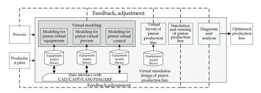
Fig. 3.13. Virtual design procedure of the piston production line
