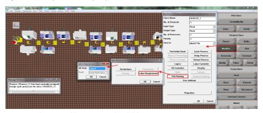
Fig. 4.5. Machine control logic associated with labor
