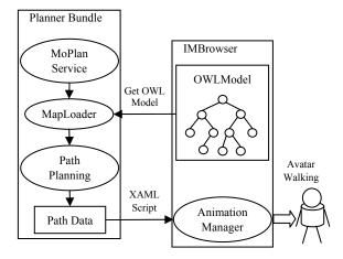
Fig. 12. The process of how to generate animations through the motion planning component
