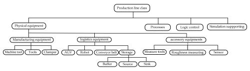
Fig. 3.4. Static hierarchy of piston production line objects
