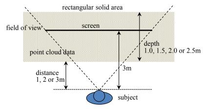
Fig. 7. Condition of experiment on representation of point cloud data.
