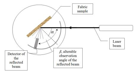
Fig. 6. Scheme of the reflection study experiment
