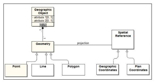
Fig. 6. A class diagram of geographic object orientation
