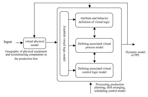
Fig. 3.11. Steps of building virtual dynamic model
