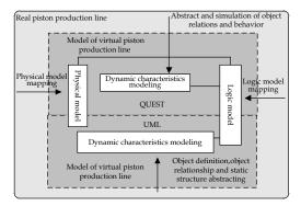
Fig. 3.2. VD-PPL simulation and modeling method based on QUEST+UML
