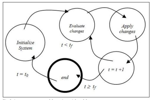
Fig. 2. A common structure of dynamic spatial models.
