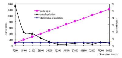
Fig. 4.12. Relationship between simulation time and cycle time
